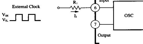
If an excessive input is applied, the OSC block may not function. In this case, connect the current limiting resistor R1.
