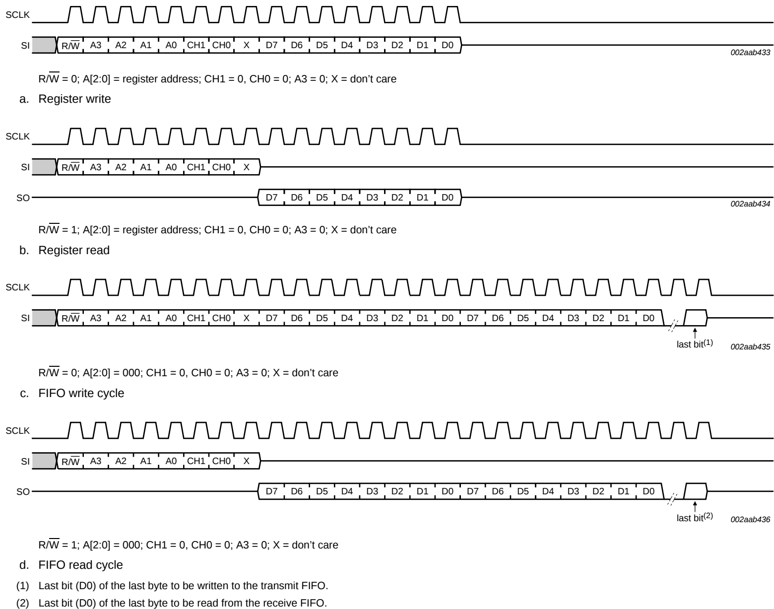
Fig 17. SPI operation
