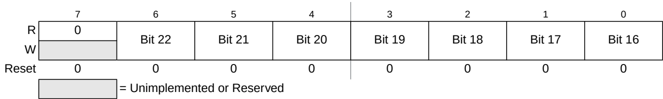
Figure 20-15. Debug Comparator Address High Register (DBGXAH)
