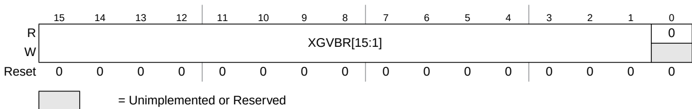
Figure 6-5. XGATE Vector Base Address Register (XGVBR)
