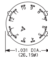
TERM. NOS. MOLDED ON HOUSING
