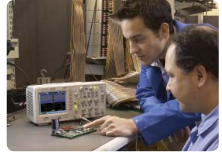
Figure 4. The bright, crisp display on the 1000 Series oscilloscope and its wide viewing angle let you quickly identify your signal activity.
