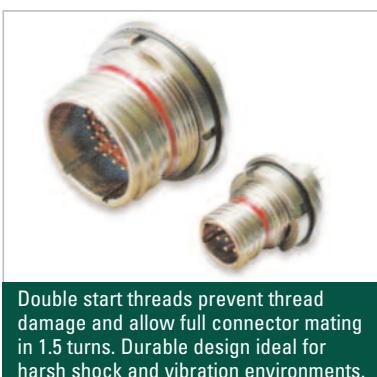
Double start threads prevent thread damage and allow full connector mating in 1.5 turns. Durable design ideal for harsh shock and vibration environments.
