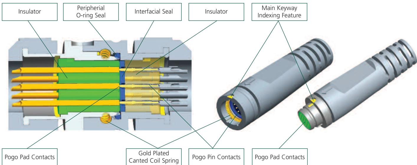
Special Pogo Pin/Pad Connector. See factory for details.
