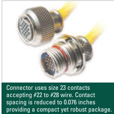
Connector uses size 23 contacts accepting #22 to #28 wire. Contact spacing is reduced to 0.076 inches providing a compact yet robust package.
