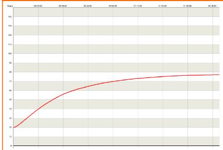
Exemplary measurement at room temperature without additional heat sink.
