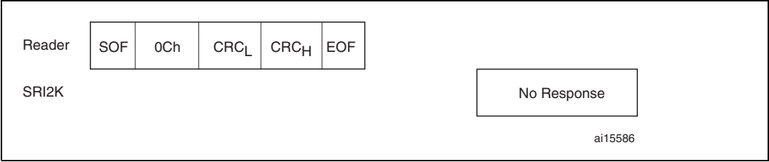
Figure 57. Reset_to_inventory frame exchange between reader and SRI2K
