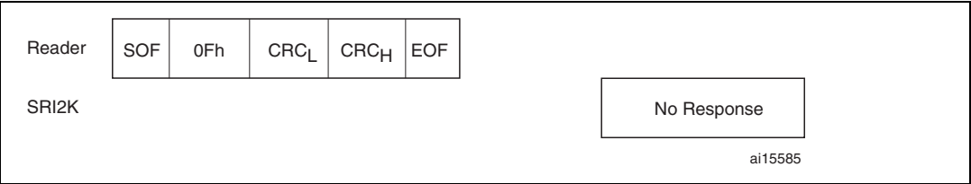
Figure 37. Completion frame exchange between reader and SRI2K
