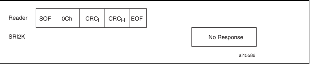
Figure 40. Reset_to_inventory frame exchange between reader and SRI2K
