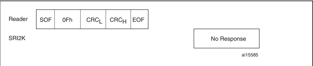
Figure 56. Completion frame exchange between reader and SRI2K
