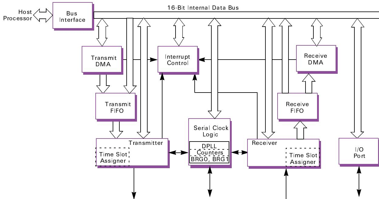
The on-chip DMA channels allow high speed data transfers for both the receiver and the transmitter. The IUSC supports automatic status and control transfer through DMA, and allows initialization of the serial controller under DMA control. Each DMA channel can do a 16-bit transfer in as little as three 50 ns clock cycles, and can generate addresses compatible with 32-, 24- or 16-bit memory ranges.
