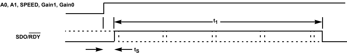
FIGURE 28. SDO/RDY DELAY AFTER MULTIPLEXER CHANGE
