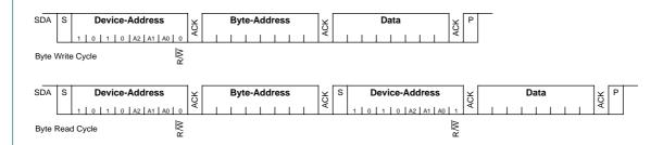
After the ASI slave IC has sent the START condition, the device address is transmitted. This address serves for the selection of a maximum of 8 possible E<sup>2</sup>PROM ICs on this bus. This device address is defined as 000 within the ASI slave IC interface. Therefore in the application the PINS AO...A2 of the E<sup>2</sup>PROM are always set at Uss of the E<sup>2</sup>PROM.
