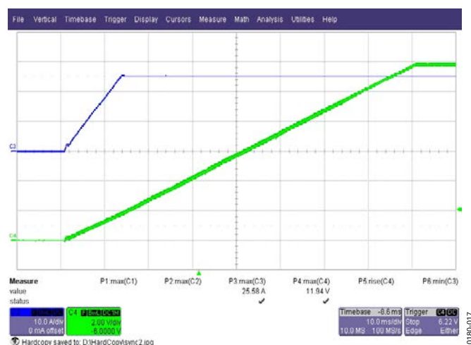
Figure 18. Startup at 385 V DC, 25 A Load (1 A/ \mu s Slew Rate) Green Trace: Output Voltage, 2 V/div, 10 ms/div Blue Trace: Load Current, 10 A/div, 10 ms/div
