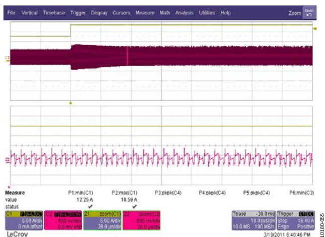
Figure 56. Input Current During Load Step of 10 A to 20 A Showing Steady Balancing of Both Phases; Yellow Trace: Load Current, 5 A/div, 10 ms/div Red Trace: Voltage at CS1 Pin, 500 mV/div (20 \mu s/div Zoomed In)
