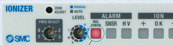
Maintenance display LED light ON
