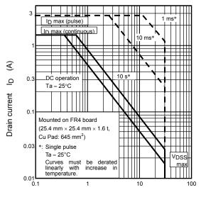
Drain-Source voltage  $V_{DS}$  (V)
