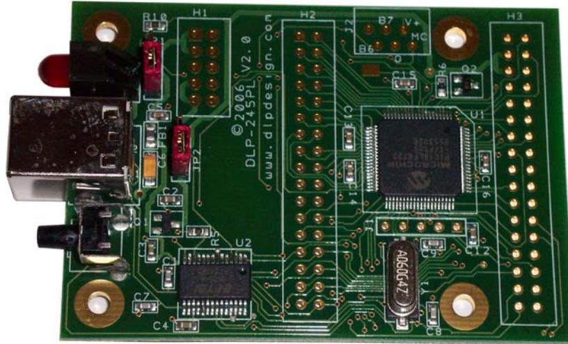
The DLP-245PL-G combines the same lead-free USB interface used in the DLP-USB245M-G module with a Microchip PIC microcontroller to form a rapid development tool. The 18LF8722 microcontroller is preprogrammed with basic functionality for accessing the port pins and can be reprogrammed with user hex code via a 5-pin header that is compatible with Microchip's MPLAB ICD2 device programmer/debugger (purchased separately).
