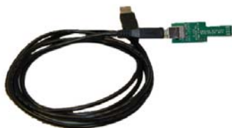
USB-TO-UART CONVERTER (ADE8052Z-DWDL1)
