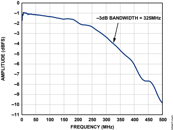
Figure 53. Full-Power Bandwidth vs. Frequency, AD9222-50
