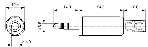
Cable diameter max. 4.0 mm
