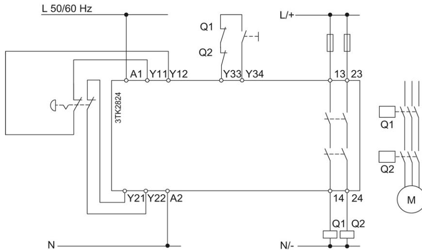
Figure 3-22 EMERGENCY STOP (2-channel) with additional ON button
