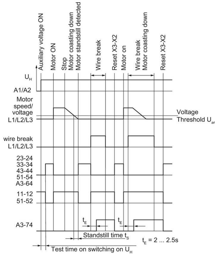
Figure 3-1  $t_E$ : Detection time after wire break
