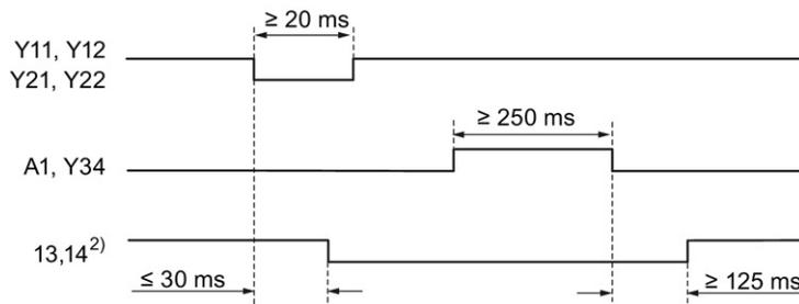
Figure 3-70 State diagram 3TK2850 / 3TK2851 / 3TK2852 monitored start
