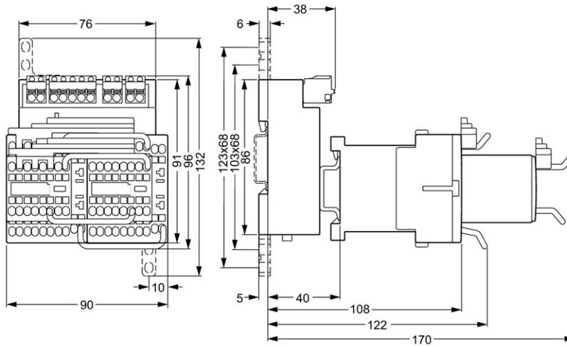
Figure 6-11 3TK2852 spring-loaded
