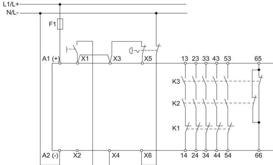
Figure 3-65 Monitored start; EMERGENCY STOP (2-channel)
