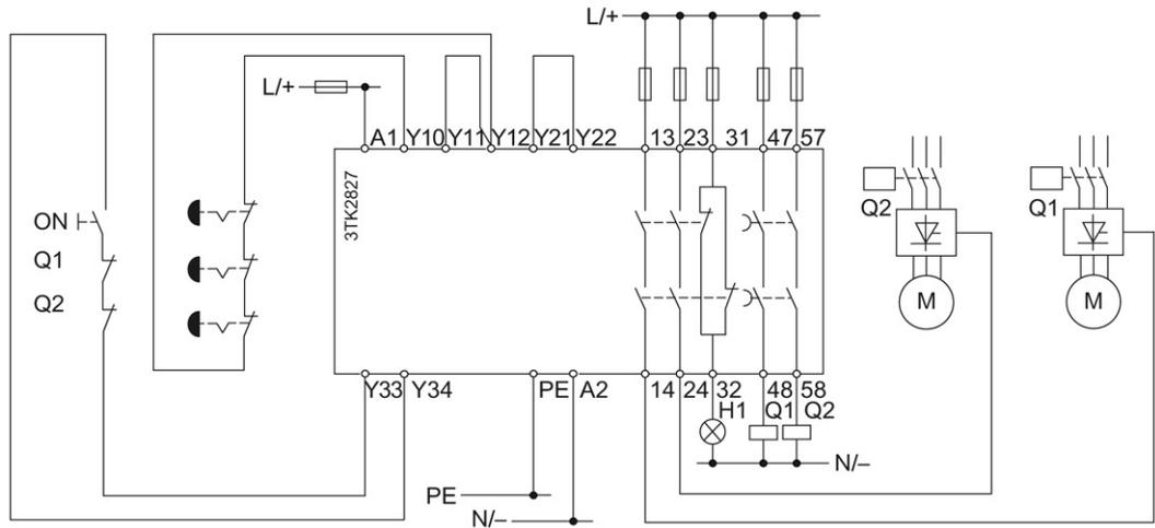
Figure 3-33 Monitored start (1-channel)
