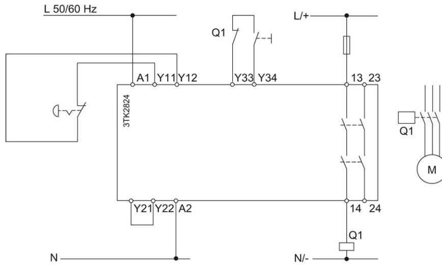
Figure 3-23 EMERGENCY STOP (1-channel) with additional ON button
