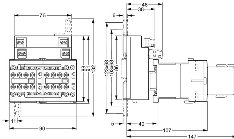
Figure 6-15 3TK2856 spring-loaded
