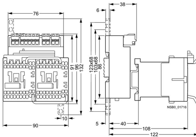
Figure 6-9 3TK2850/51 spring-loaded
