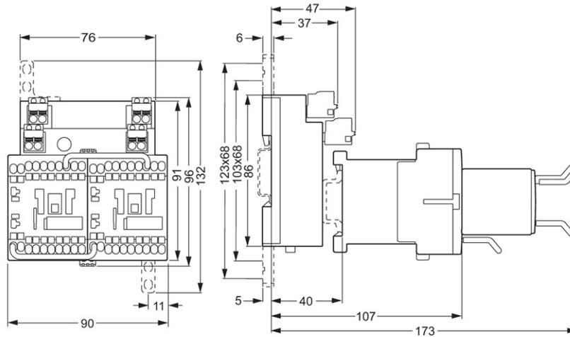
Figure 6-17 3TK2857 spring-loaded
