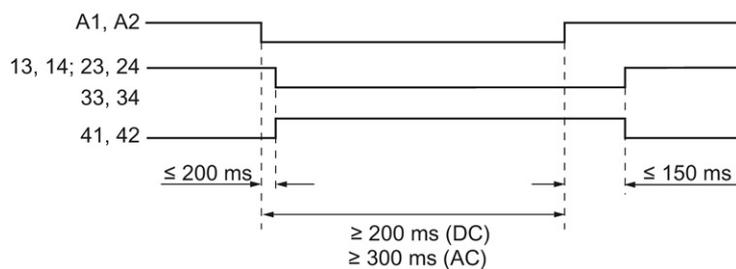
Figure 3-14 State diagram 3TK2821/24
