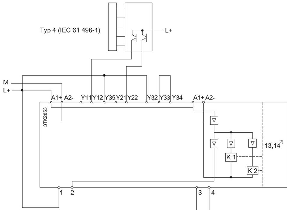
Figure 3-82 Light array monitoring (2-channel) without cross-circuit detection
