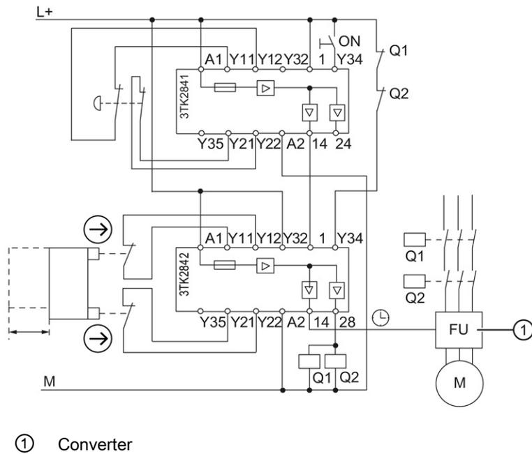
Figure 3-63 Cascading, EMERGENCY STOP + protective door monitoring, (2-channel)
