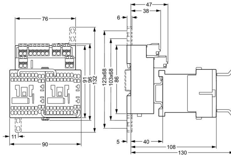
Figure 6-13 3TK2853 spring-loaded
