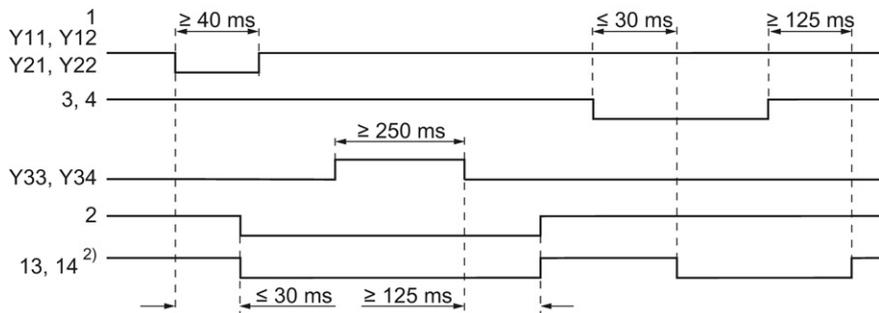
Figure 3-77 State diagram 3TK2853 monitored start
