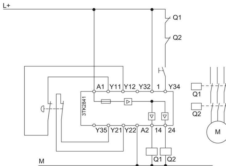
Figure 3-51 Monitored start (2-channel)
