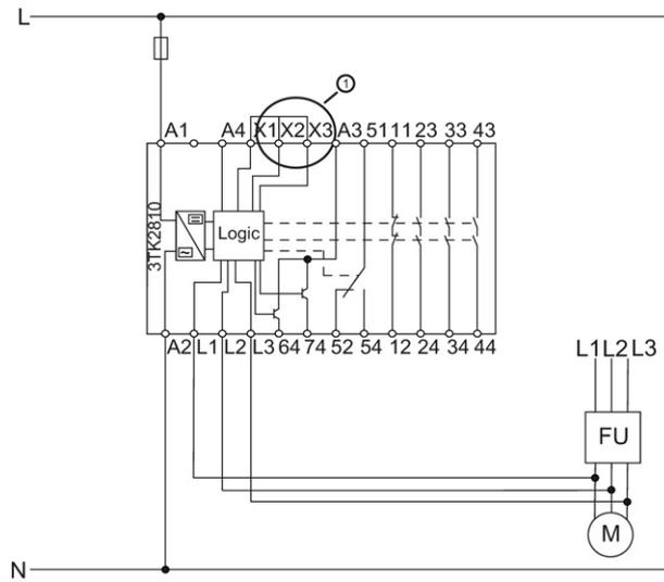
① With jumper between X2-X3 for automatic acknowledgment of open-circuit detection
