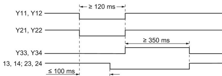
Figure 3-20 State diagram 3TK2824-.A.
