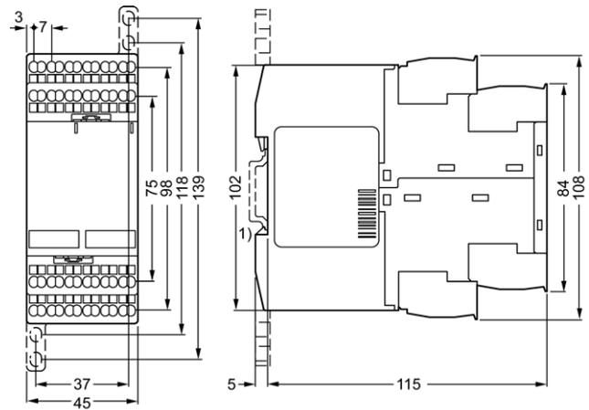
Figure 6-2 3TK2810/25/26/27/28/34/45 spring-loaded
