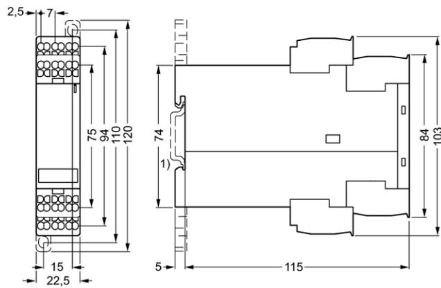
Figure 6-5 3TK2821/22/23/24/30 spring-loaded
