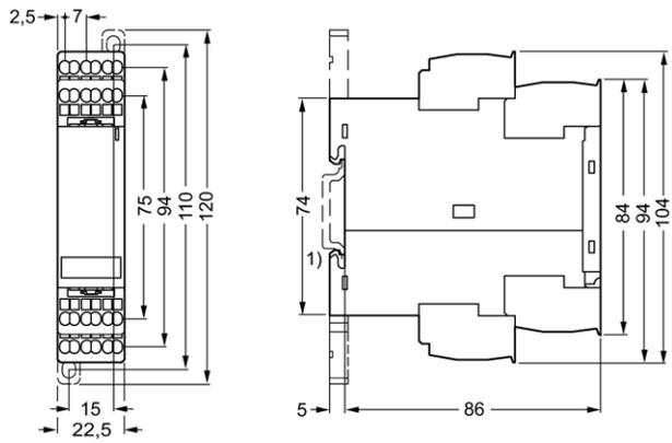
Figure 6-7 3TK2840/41/42 spring-loaded
