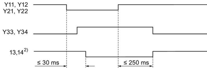
Figure 3-69 State diagram 3TK2850 / 3TK2851 / 3TK2852 autostart
