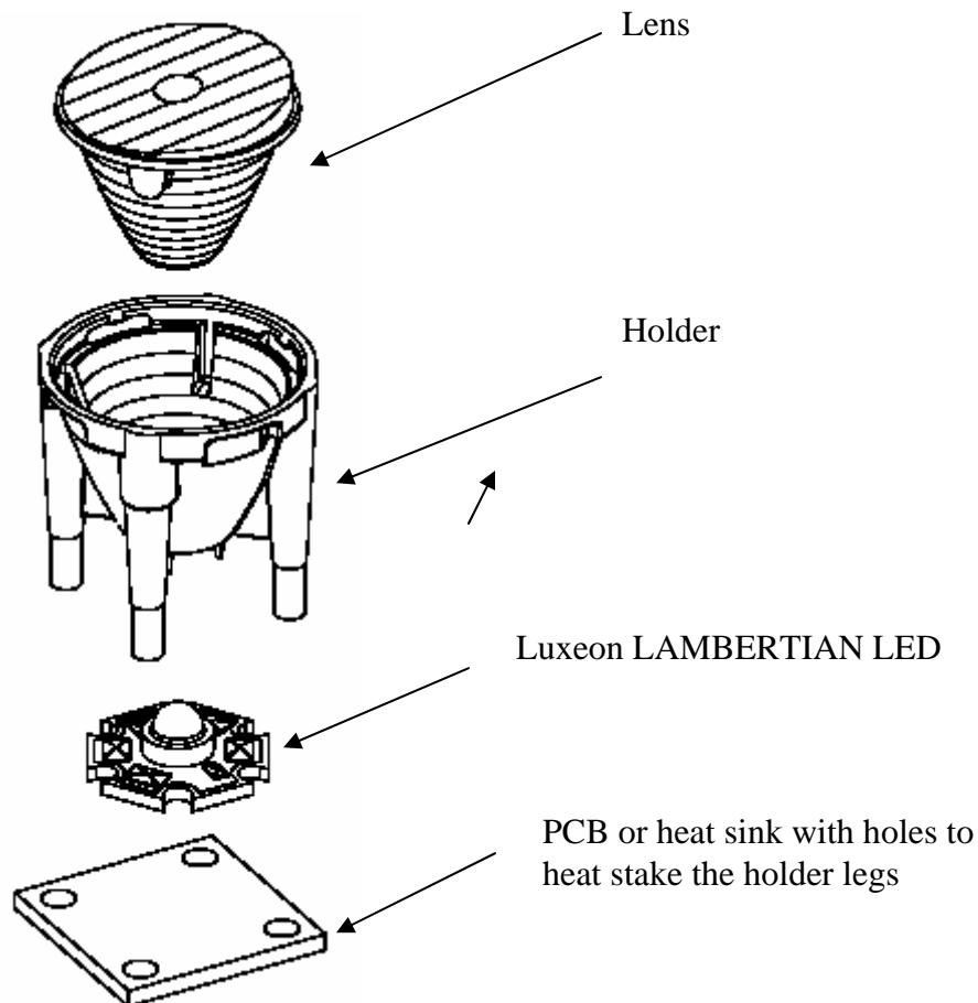
Note: If using a Lambertian Luxeon™ LED and a Fraen lens without a lens holder, a "Spacer Ring" is required to achieve the correct distance between the Luxeon™ LED and the lens. Further information about Spacer rings is available below (Section "Spacer Rings, Usage").
