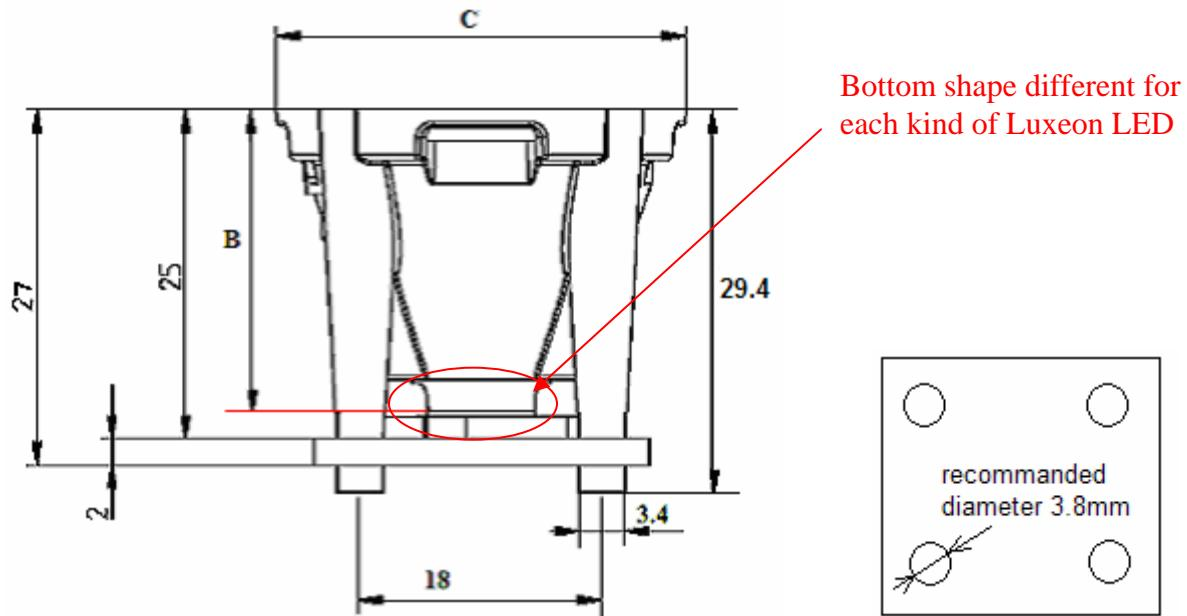
To achieve the correct distance between any Lambertian Luxeon LEDs and the lens, specific holders have been designed. They can be recognized by their interface:
