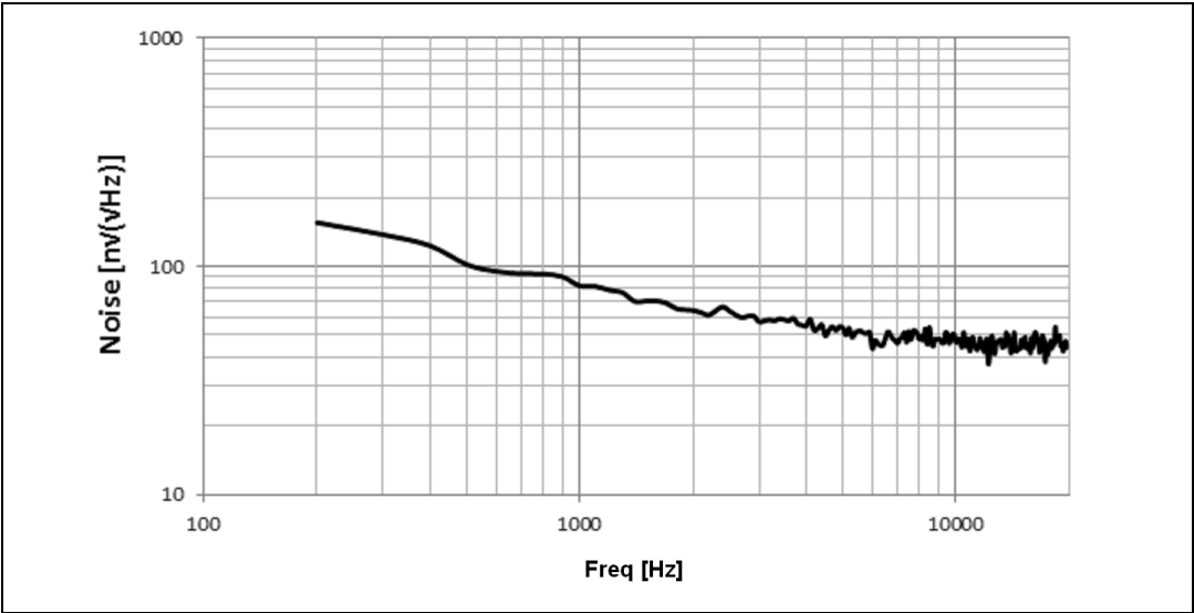
Figure 38. OPAMP voltage noise versus frequency
