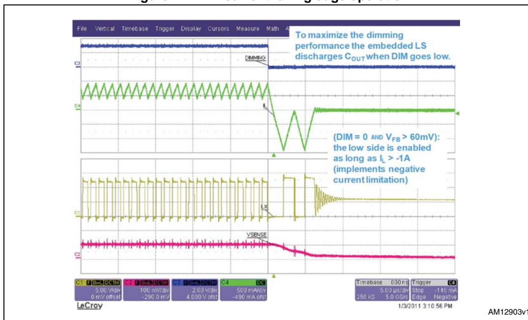
Figure 12. LED current falling edge operation
