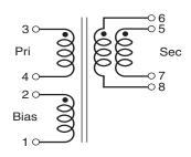
Secondary windings to be connected in parallel on the PC board
