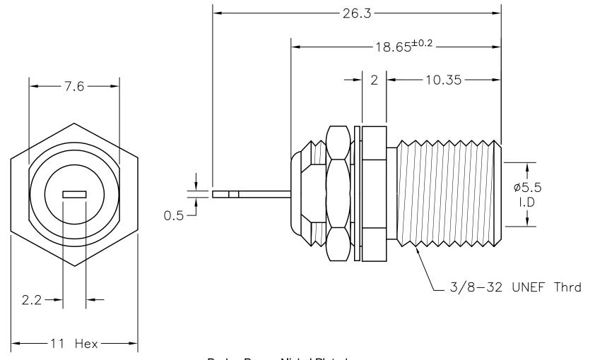
Body: Brass, Nickel Plated Contact: Brass, Nickel Plated
