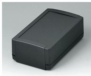
B1070369 TOPTEC 194 H, Vers. I ABS (UL 94 HB) black RAL 9005 7.64"x4.53"x2.68" IP 40
