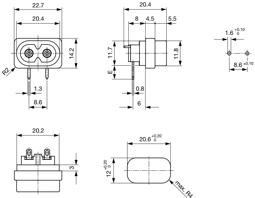
E = PCB terminal standard (additional solder): 6.8 mm
