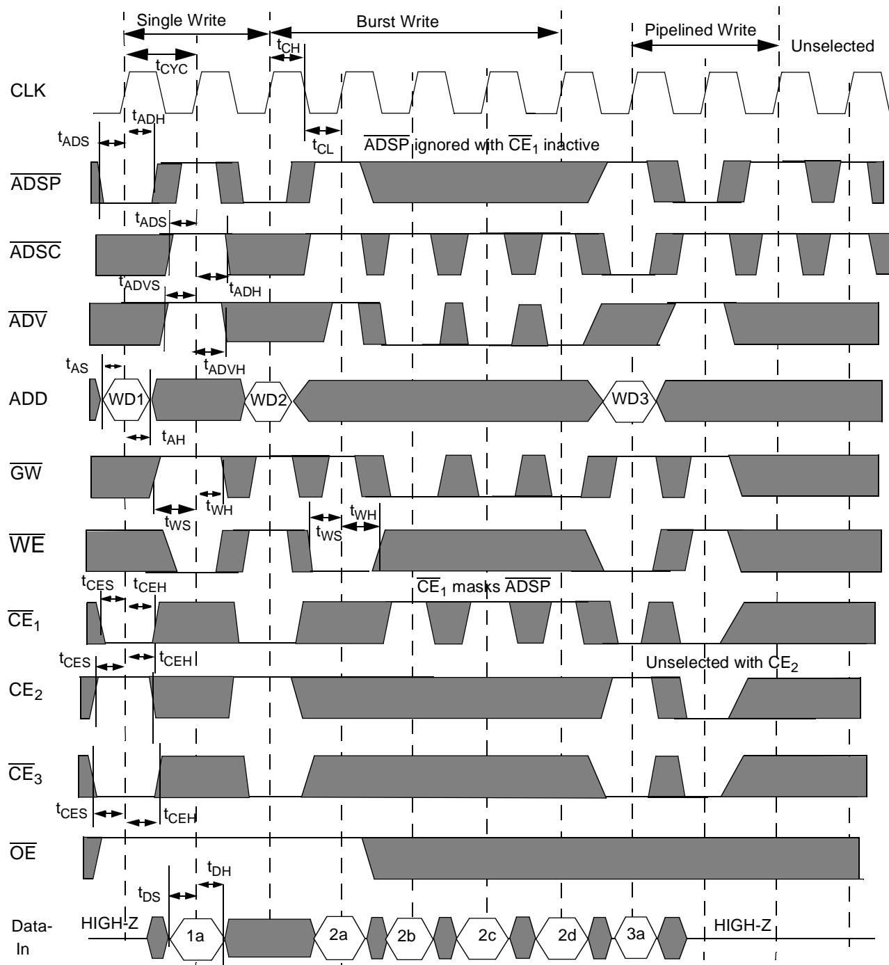
$\overline{WE}$  is the combination of  $\overline{BWE}$  &  $\overline{BW}_x$  to define a write cycle (see write cycle definition table).
