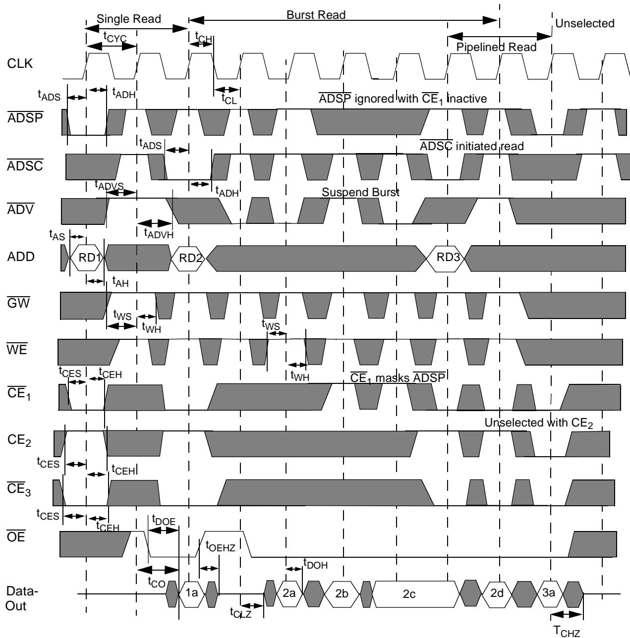
**WE** is the combination of **BWE** & **BW<sub>x</sub>** to define a write cycle (see write cycle definition table).
