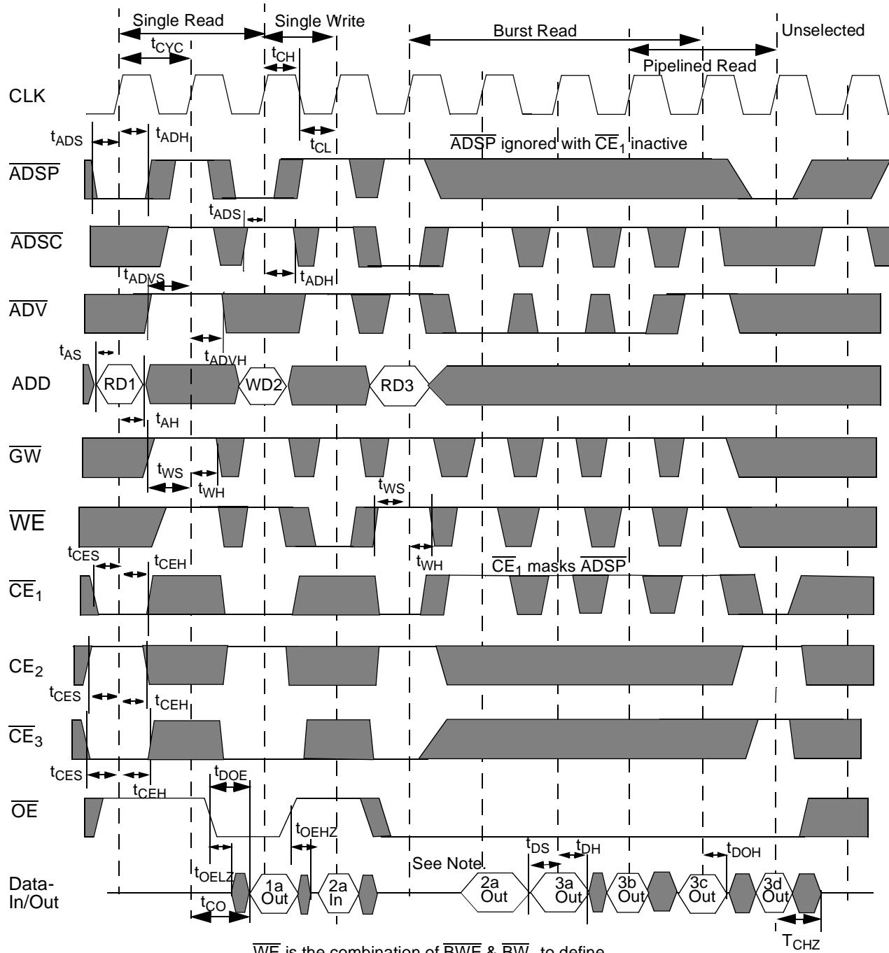
WE is the combination of  $\overline{BWE}$  &  $\overline{BW}$  to define a write cycle (see write cycle definition table).
