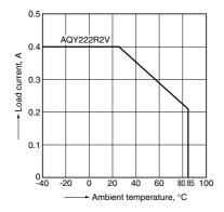
1.-(2) Load current vs. ambient temperature characteristics
