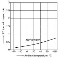
6.-(2) LED turn off current vs. ambient temperature characteristics Load voltage: 10V (DC);
