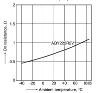
2.-(2) On resistance vs. ambient temperature characteristics
