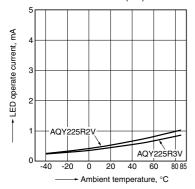
6.-(1) LED turn off current vs. ambient temperature characteristics Load voltage: 10V (DC);
