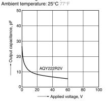
12.-(2) Output capacitance vs. applied voltage characteristics
