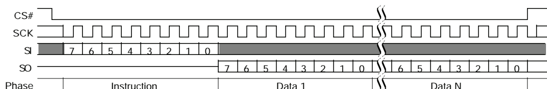
Figure 10.70 Password Read (PASSRD E7h) Command Sequence
