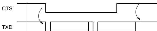
Figure 30-19. Transmitter Behavior when Operating with Hardware Handshaking
