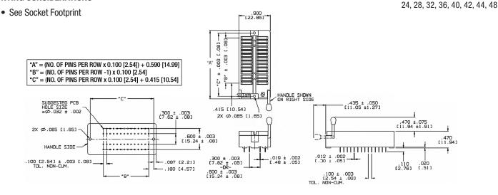
**ALL DIMENSIONS: INCHES [MILLIMETERS]** ALL TOLERANCES: ±0.005 [0.13] UNLESS OTHERWISE SPECIFIED FOR TEST SOCKET RECEPTACLES, SEE DATA SHEET 10003 DO NOT USE THIS SOCKET IN A BURN-IN OVEN WITH CONTACTS IN OPEN POSITION, AS IT WILL DAMAGE THE SOCKET **CONSULT FACTORY FOR OTHER SIZES AND CONFIGURATIONS**
