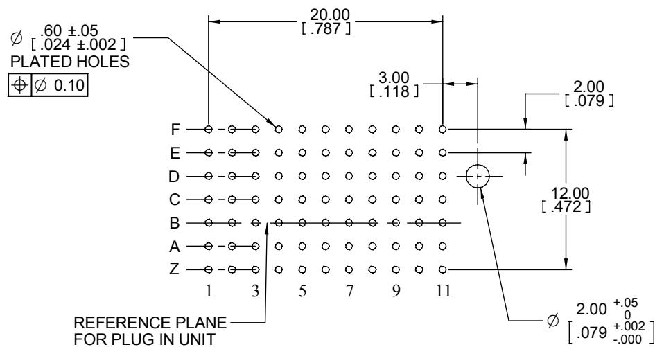
Recommended PCB hole mounting pattern
