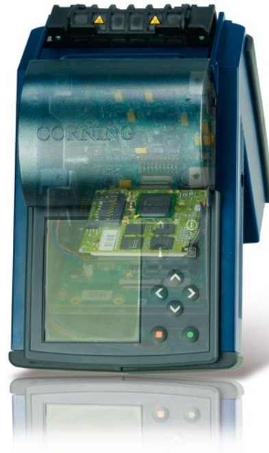
CORNING Cable Systems GmbH: glass fiber splicing unit PHYTEC contribution: development of customized hardware, application of standard modules
