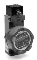
Hazardous environments demand Honeywell. When conditions are hazardous and performance is critical, Honeywell Sensing and Control (S&C) delivers exceptional performance. Our hazardous location switches are limit switches designed specifically for dangerous indoor or outdoor locations — where reliability and repeatability are essential. To comply with explosion-proof requirements, the flame path within the switch housing is designed to contain and cool escaping hot gases
