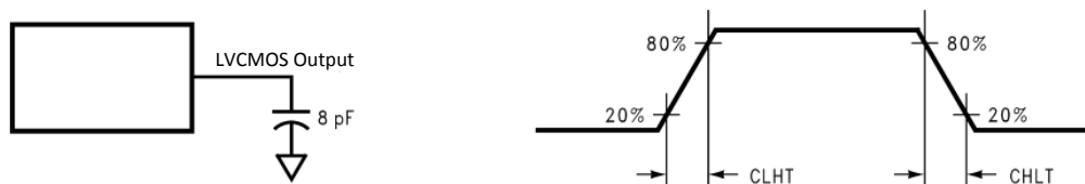
Figure 2. LVC MOS Output Load and Transition Times
