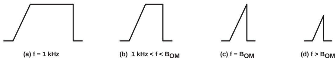
Figure 5. Full-Power-Response Output Signal
