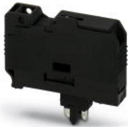
Fuse plug, fuse type: Sand filled, connection method: Plug connection, nominal current: 10 A, nom. voltage: 500 V, width: 8.2 mm, fuse type: G / 5 x 20, color: black
