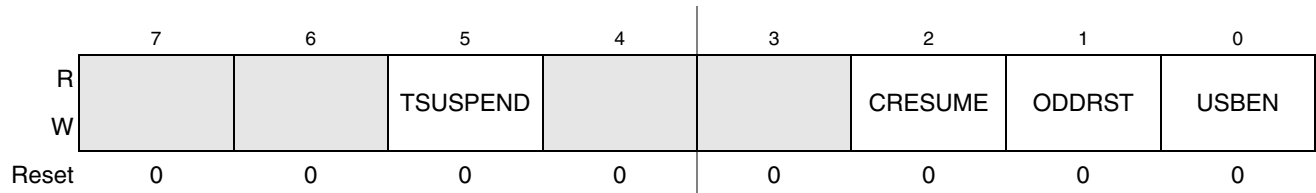
Figure 17-13. Control Register (CTL)
