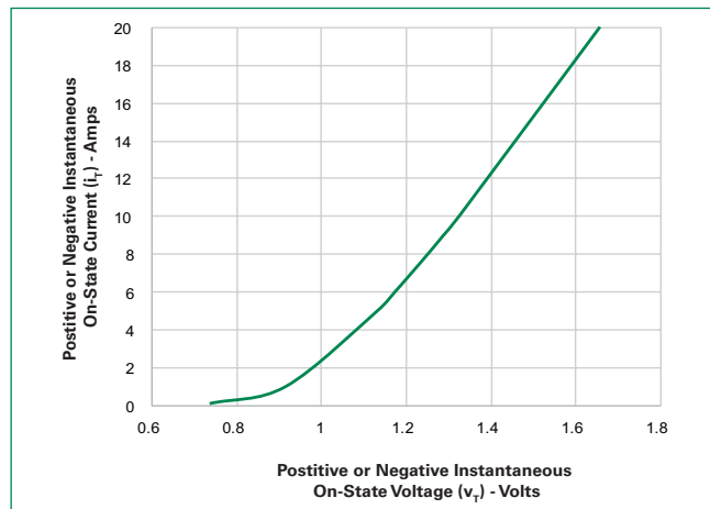
Figure 7: On-State Current vs. On-State Voltage (Typical)
