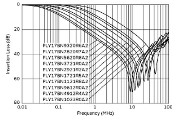
Differential Mode Insertion Loss-Frequency Characteristics
