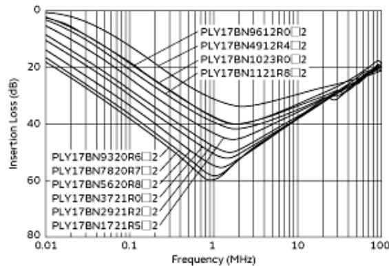
Common Mode Insertion Loss-Frequency Characteristics
