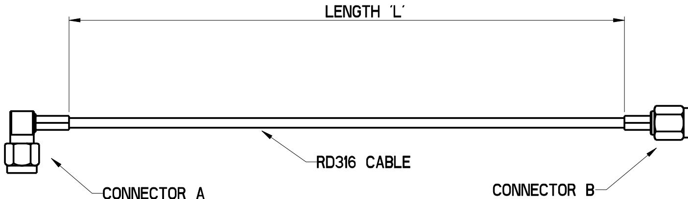
FIT 25mm HEAT SHRINK SLEEVE AT EACH END
