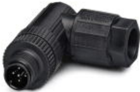
Connector, 5-position, Plug angled M12, A-coded, Spring-cage conn., Knurl material: Plastic, External cable diameter 4 mm ... 8 mm
