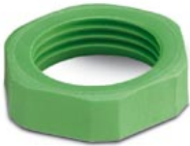
Nut (plastic) to lock the contact carrier Pg13.5 / 27 WAF
