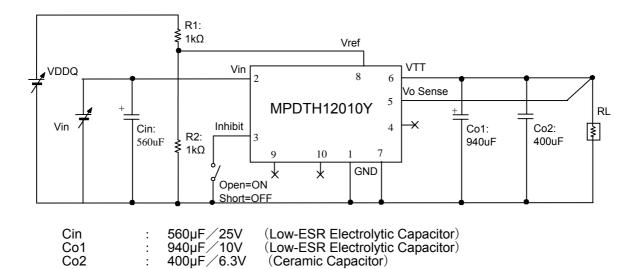
Ripple Noise Measurement Circuit
