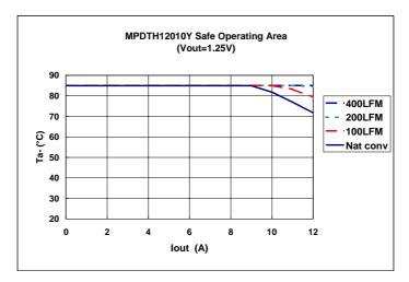
The above SOA represents the condition at which internal components are at or below the manufacturer's maximum operating temperatures. Derating limits apply to modules soldered directly to 4 in.×4in. 4 layer PCB with 1 oz. copper. For more reliable operation, appropriate derating is desirable.
