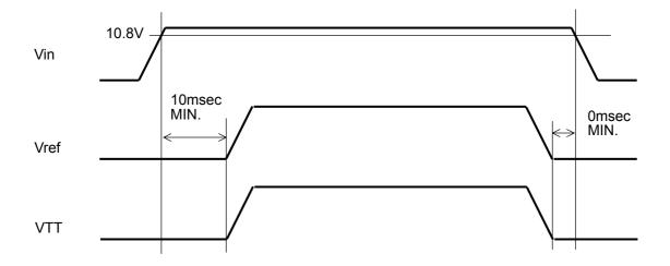
(2) Start-up using Inhibit pin
