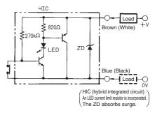
Note: The load may be connected to either the +V or 0 V terminal. Core wire colors have been changed accompanying changes in standards. The old core wire colors are given in parentheses.
