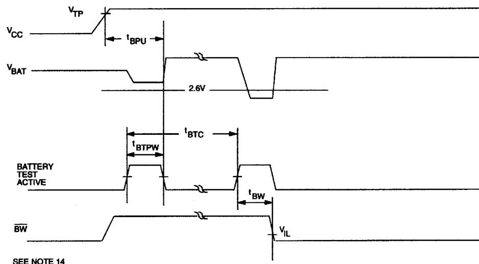
**POWER-DOWN/POWER-UP TIMING** (t<sub>A</sub>: See Note 10)
