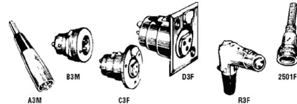
Plugs and receptacles offer up to 5-contact versatility by means of up to four circuit contacts plug electrically integrated ground terminal on shell. Neoprene cable strain relief bushing keyed to shell; ribbed for easy access to male plugs. Die-cast zinc alloy with satin-nickel finish. Receptacles will mate with all standard audio connectors. Right angle configuration reduces "cable clutter."
