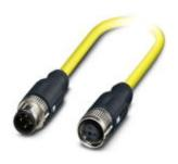
Sensor/Actuator cable, 4-position, PVC, Yellow RAL 1021, shielded, Plug straight M12-SPEEDCON, A-coded, on Socket straight M12-SPEEDCON, A-coded, Cable length: 0.5 m
