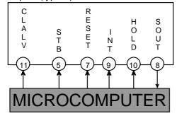
This type uses CLALV,STB,RESET,INT,HOLD,SOUT terminal as I/F terminal to the microcomputer. This is the typical type at M52957AFP.
