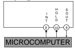
This type does not connect CLALV,STB,RESET terminals to the microcomputer.
