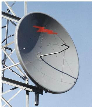
4.6 m | 15 ft Standard Parabolic, Low VSWR Unshielded Antenna, single-polarized, 6.425–7.125 GHz, PDR70, gray antenna, with flash, standard pack—two-piece reflector
